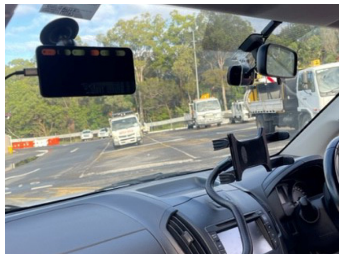
Image: Positioning of Retina Visions camera that is attached to the internal windscreen of the back loggers vehicle and requires no manual interaction. Installation of the Retina Visions camera takes less than 10 minutes.
