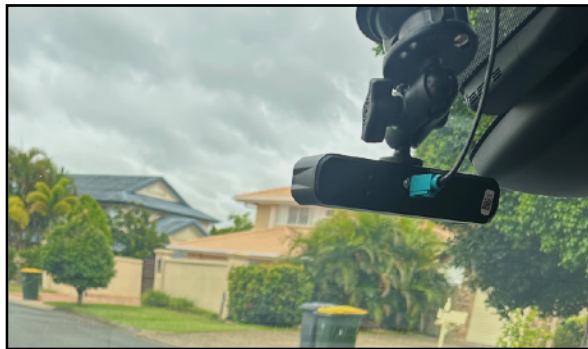
Road asset data is collected by dash-mounted cameras on any council or contractor vehicle (waste collection, street sweepers, utility etc)
